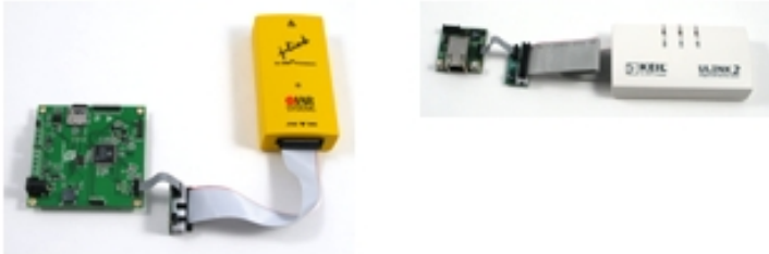
10-pin to 20-pin JTAG Adapter used with a Stellaris LM3S811 evaluation kit to debug a Stellaris Serial-to-Ethernet module (MDL-S2E)
